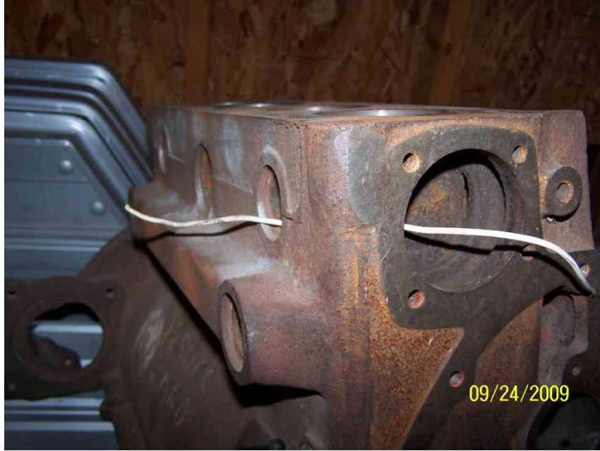
These next photos were taken to show that the block, with the exception of the piston cylinders is basically hollow and water is free to circulate (or stand) freely within it.
