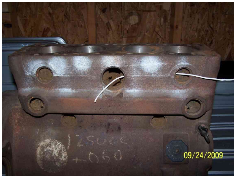
These next photos were taken to show that the block, with the exception of the piston cylinders is basically hollow and water is free to circulate (or stand) freely within it.
